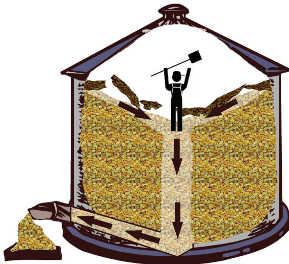
Figure 6. Moldy bridge has broken causing person to fall into the void and flowing grain.
