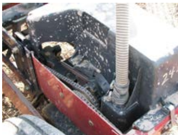
Figure 1. Sprockets, bearings, chains, and other moving parts should be evaluated for wear and serviced according to the manufacturer's manual.
